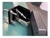
2. Gently insert the male connector plug from the sensor unit into the main unit's female socket, and hand tighten the locking nut. Please do not use excessive force or any pliers or spanners to tighten this nut. This nut is an IP68 rated connector, so there is no need to use extra sealant around this connector or over-tighten it.
