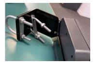
2. Install the Water Pressure Sensor (as per image on the right) onto a chosen point on the pipe.
